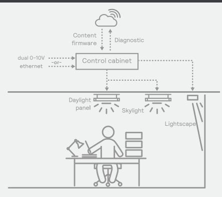
In larger installations the NatureConnect system can be integrated with an external lighting control system.
